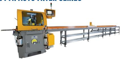
PMI Auto Miter Series are fully automatic saws. These high speed circular saws have automatic saw head rotation and material indexing. Features include touchscreen control for easy job setup, servo motor driven pusher system (available in working lengths from 14-3/4' to 35', shorter or longer lengths are available by request) and saw head rotation, fully automatic saw cycle, and program storage.
