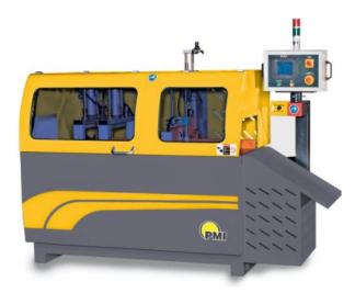
The PMI-455 A-Type is designed for sawing Aluminum Extrusion and Other non-ferrous metals. The saw's powerful 10 HP saw motor allows it cut quickly and accurately. The PMI-455 A-type's ballscrew/servo-controlled material indexing system ensures accurate, precise, and repeatable cut lengths.
