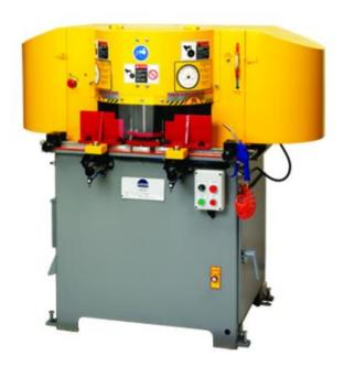
The PMI-14 B-Type is a 45 Degree Double-Blade Sawing Machine for making framing and notching cuts of non-ferrous material quickly, accurately and with a burr free finish. It has two saw blades that are positioned at 45 degrees vertically to reduce waste. The PMI-14 B is ideal for manufacturers of door and window frames because it produces two opposing 45 degree cuts in a single cycle. The double saw blade design greatly increases production and efficiency.
