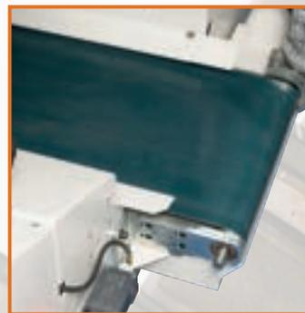
Chip belt conveyor for optimal cleaning of the working area.
