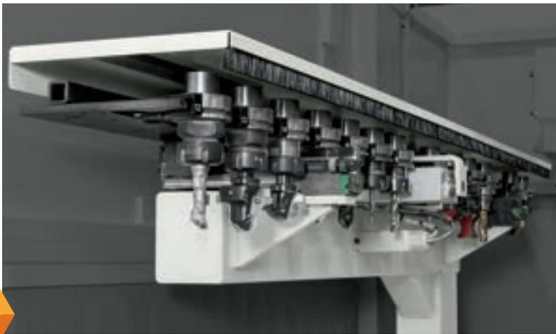
ST 14 PLUS: tool changer inside the protective structure that ensures maximal productivity and a quick set-up.
