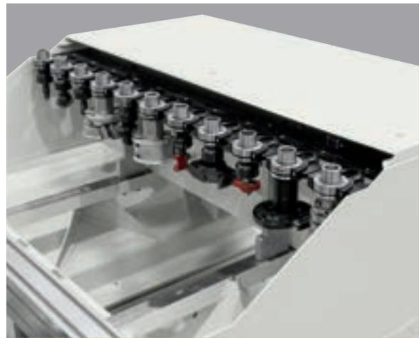
LINEAR 11: linear tool changer on the structure for management of large dimensioned tools.
