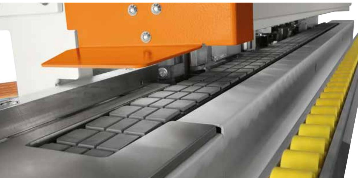
Linear and perfect feed thanks to feeding chain track with high grip rubber coated pads and sliding on industrial chain. High resistance to lateral loads thanks to special guides with one circular section and one flat section.
