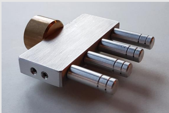
(I) Dowel nozzle with 4 pins, each pin with double glue delivery
