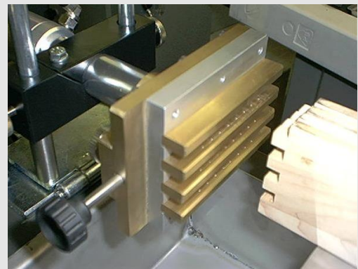
(H) Glue application for one set at a time with the 4 sides of the drawer
