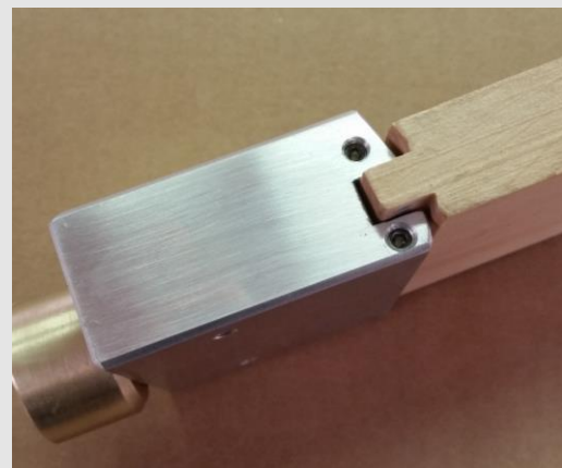
(B) Nozzle for coped profiles for 5 parts cabinet doors
