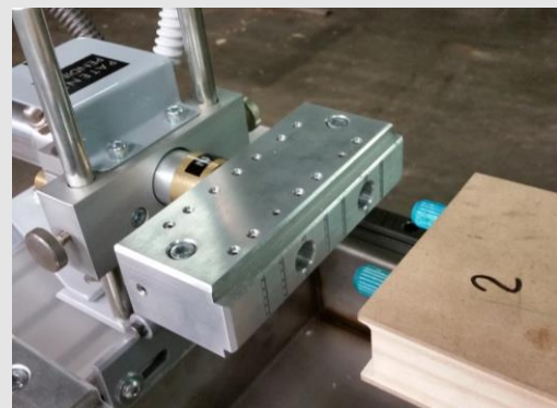
(L) Opposite dowel nozzle for glue application around the dowels
