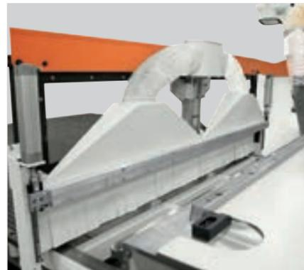
Unloading device with integrated suction system (optional)
