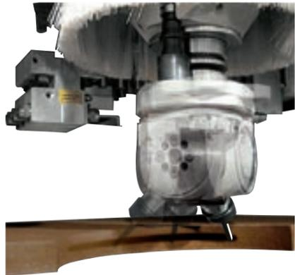
0 ÷ 360 unit: flexibility without limits. Unit with digital control managed by numerical control for positioning at 360° of the angular aggregates. (optional)
