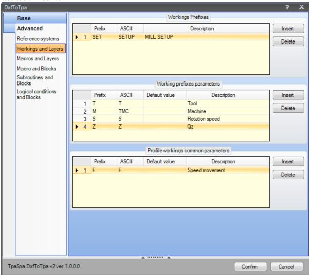
In the first list the prefix SET is associated to the working which has the ASCII name "SETUP" and description "MILL SETUP". Regarding this working are defined the parameters (second list):
