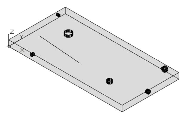
The parallelepiped which draws the piece is defined with a polyline and it corresponds to the piece layer: it defines the 3 dimensions, particularly the thickness on the Z direction.
