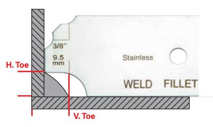
Slide the gauge so it rests against the upright vertical metal piece. The end of the gauge should make contact with the horizontal metal piece. If there is space between the gauge and the horizontal toe of the weld, then the weld is undersize. Check the vertical toe as well. The vertical scribe lines will show where the vertical toe should be.
