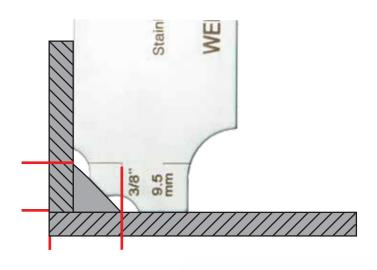
The protusion in the middle of the gauge should make contact with the weld to verify that it is not concave. If there space between the protusion and the weld, it is not an acceptable fillet. Welds should never be concave.
