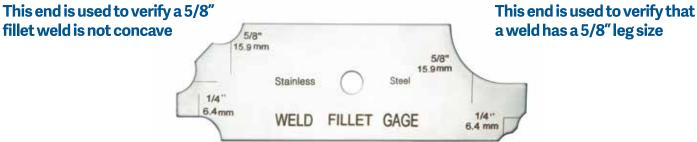
This end is used to verify that a weld has 1/4" leg size
