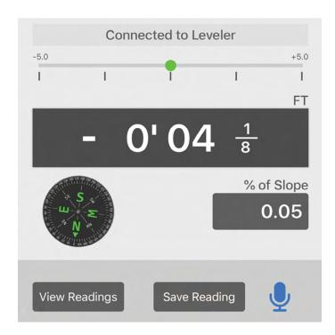
Advanced functions include- % of Slope, Range where you set the acceptable tolerance and have audible and light indications as well as the readings, save photos and comments with your readings with the press of a button, and more.
