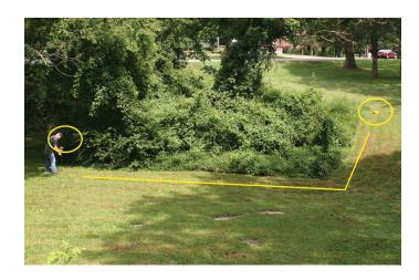
There is no setup time. Just set the reel on its side and as quickly as you can walk and set the readout down you have a valid reading. No clear line of sight needed- works around or behind obstructions. One man operation.
