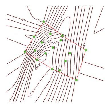
3D Terrain and Structure Mapping. No other instrument on the market can create a true X,Y,Z formatted survey in real time on the job site. Perfect for upload into CAD\*. \*CAD programs not included.
