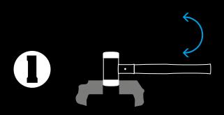
Firmly clamp the used insert in a vice and loosen with a lateral twisting movement.
