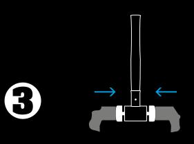
In the vice, press the new insert into the housing and insert retaining pins.
