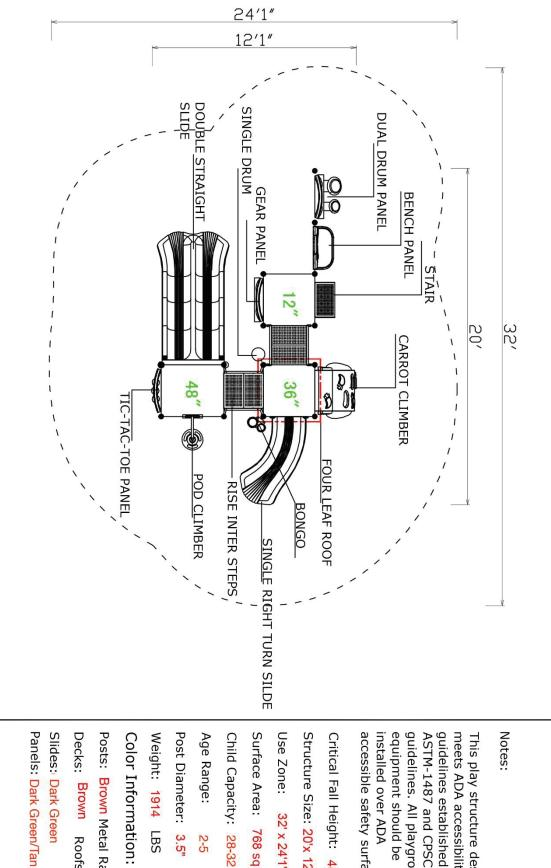
guidelines. All playground guidelines established in Decks: Brown Roofs: Green/Tan Surface Area: 768 sq ft Structure Size: 20'x 12'1"x 10'7" accessible safety surfacing meets ADA accessibility Posts: Brown Metal Rails: Tan Use Zone: 32' x 24'1" Critical Fall Height: 48" ASTM-1487 and CPSC This play structure design 2-5
