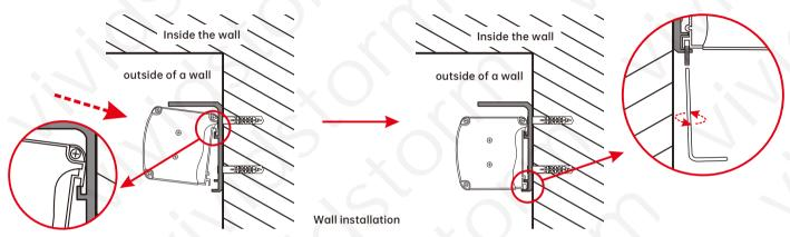
4. After the equipment is stuck in the bracket, please use the mini "L" type screw driver to tighten the screw to fix the housing and the bracket.
