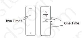
After confirming the height, use a pointed tool to press the 'Function' key on the back of the remote control 2 times. Within 10 seconds, press the 'Down' key on the remote control 1 time. The lower axis of the screen will jitter once, indicating the successful lower limit setting. Fully close and then reopen the screen to ensure the correct screen height.
