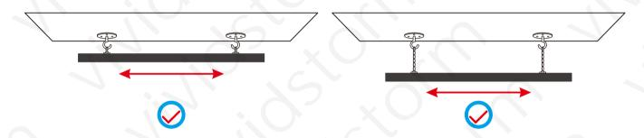
Note: please make sure the equipment is installed horizontally and do not tilt it.
