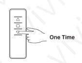
Enter adjustment mode: Use a pointed tool to press the 'Function' key on the back of the remote control 4 times, then within 10 seconds, press the 'Down' key on the remote control 1 time. At this point, if the lower axis of the screen jitters once, it indicates entry into the limit adjustment state.
