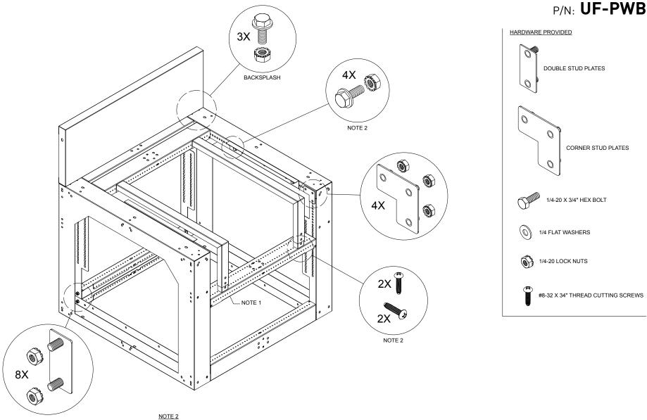
THIS HORIZONTAL CHANNEL CAN BE TURNED VERTICALLY TO MINIMIZE ACCESSORY OPENING IF NEEDED
