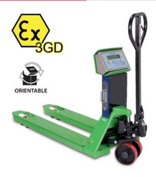
ATEX pallet truck scale for use in areas classified as hazardous (ZONE 2 and 22) with type of protection in accordance with Ex II 3G IIC T6 Gc X and Ex II 3D IIIC T115C° Dc X. Available in approved version for legal-for-trade use. Manufactured, calibrated and adjusted in Italy by Dini Argeo, using certified sample masses.
