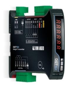
Specific weight transmitter ideal for dynamic and/or robotic high-speed weighing systems. Thanks to its algorithm and high-speed conversion rate, it calculates the weight of a package running on a weighing conveyor and store data in a memory that can be read from fieldbus. Designed for a throughput of over 200 pcs/min.
