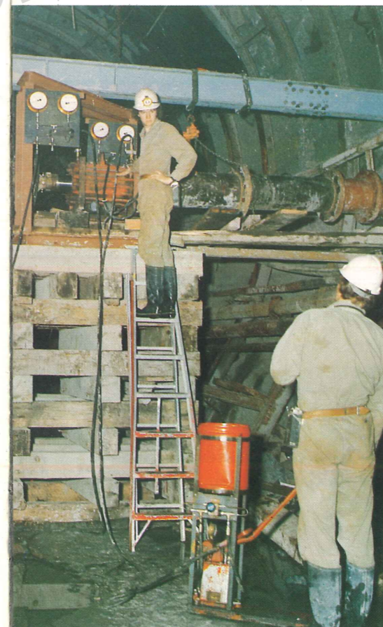
(Below) Stress measurement. Geomechanical Engineers make plate bearing tests at sides of tunnel. (Right) On location. Filming of the Authority's second documentary, "Action Loop", released in June.
