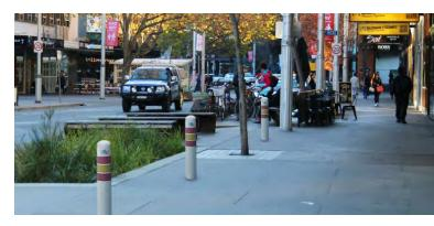
Our Energy Absorbing Bollards are approved by Transport Canberra and City Services and are compliant to Australian Road Safety Barrier System standards in AS/NZS 3845 (1999) putting it at the forefront of traffic, pedestrian and road safety solutions.
