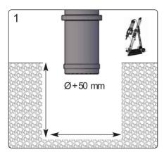
Dig a hole for the bollard instalation. Preferably with diamond bit drill, failing with jackhammer or rotary.
