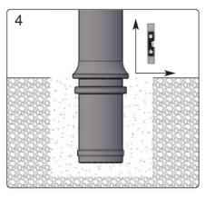
Level the bollard correctly.
