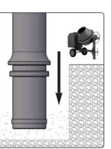
Introduce the bollard inside the hole and filled with concrete.
