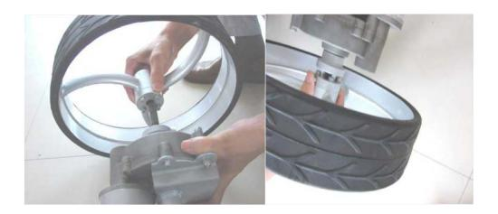
Arrange Axle assembly with drive motor to your left.
