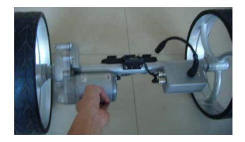
• Place trolley frame forward of the axle assembly as shown. Align mounting grooves and slide frame onto axle assembly.
