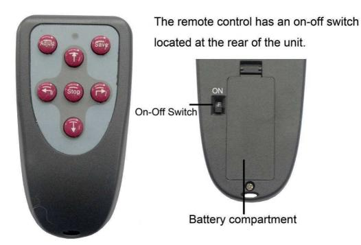
Once the cart has been turned on manually (see above) you can control the speed and direction by using the Remote Control. To initiate remote control, switch on the transmitter, turn the cart on manually and then press a button on the remote control within 3 seconds. Once the cart begins to move, the system is initiated and will remain so until the cart is switched off.
