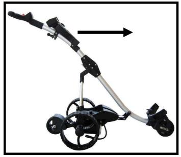
Ensure that the locking catch is fully engaged by pulling the upper part of the catch outwards if necessary. Pull down the upper bag support.
