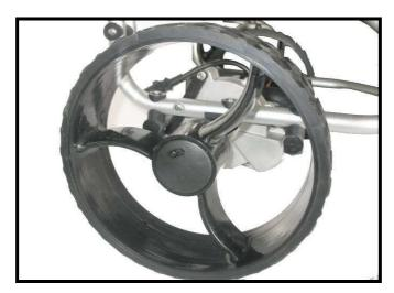
When the battery indicator is red and the voltage is too low to operate the cart (below 10.8 volts) the controller will cut power supply to the motors. In order to push the cart manually it is necessary to move the wheels out by one notch on the drive axle (freewheel position).
