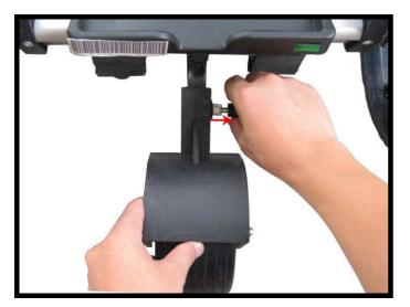
Pull spring bolt then install support wheel
