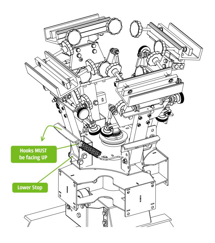
Install the upper stop bolts and rubber sleeves. Two 9/16" wrenches are required for this step. **DO NOT OVERTIGHTEN THE BOLTS**. This will cause resistance in the print head hinge point. Repeat this step for the remaining print head assemblies.
