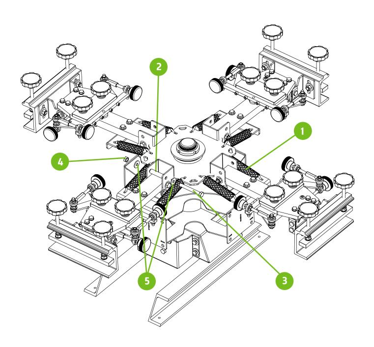
Mount the press base to a sturdy table top (2) with supplied mounting screws (1). Press is shown mounted on a Riley Hopkins 2-station press cart (sold separately). A Phillips screwdriver is required for this step.
