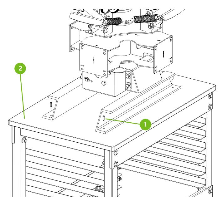
Install the print stations with supplied hardware. Ensure the number on the print station matches the number on the center rotary. Failure to due so, will shift the platens out of alignment. Do not fully tighten at this time. They must be snug, but loose enough to adjust with bumps of the hand.
