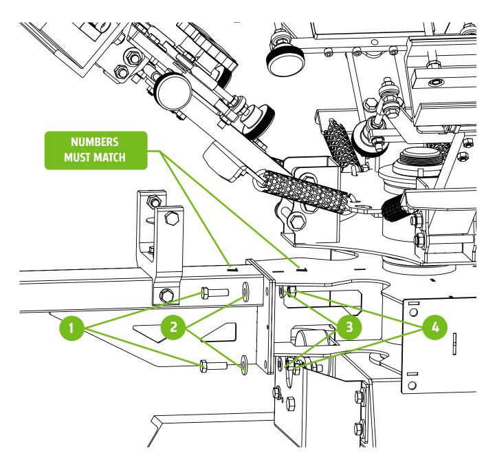
Install the 3/16" roll pins to locate the print station. Tap print station to align holes visually as close as you can. This is a factory setting that ensures your platens are aligned to each other. Tap them in approx. 1/2" with a hammer. After pins are seated, fully tighten the print station hardware.
