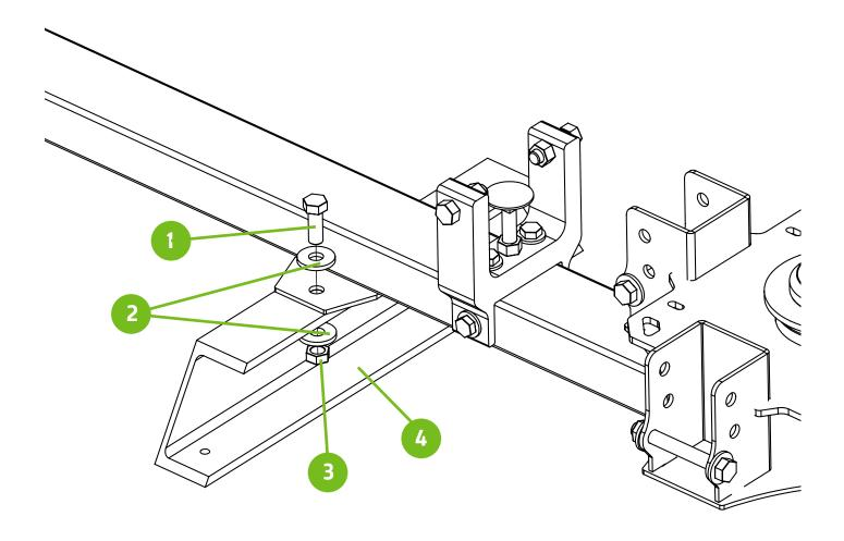
Install the Print head assemblies with the supplied hardware. Two 9/16" wrenches are required for this step. Repeat this step for the remaining print head assemblies.
