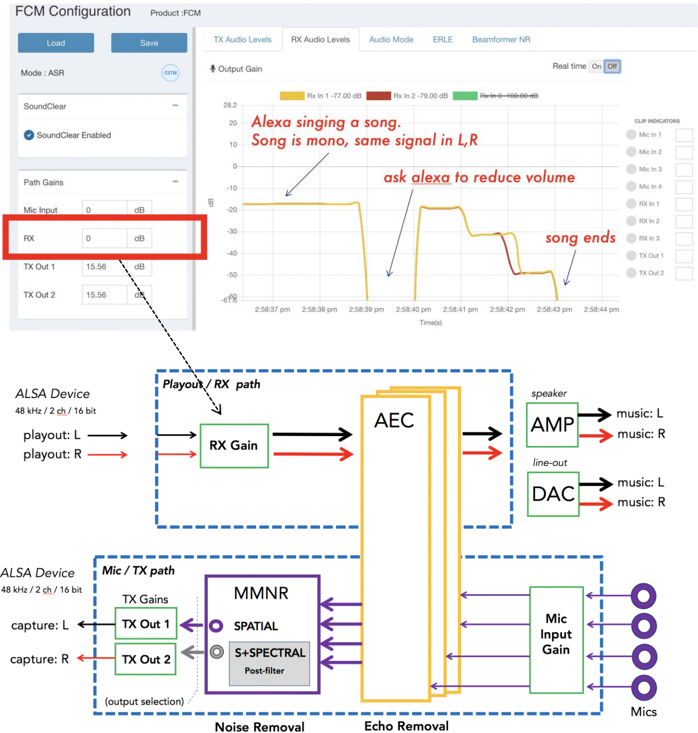
Figure 8 RX Audio Levels – Music and Responses from Alexa, and SCFF Block Diagram
