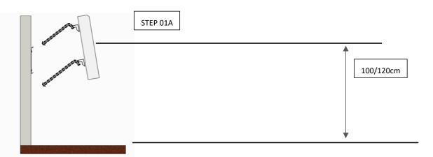
The Bracket must be installed on a flat and vertical wall.
