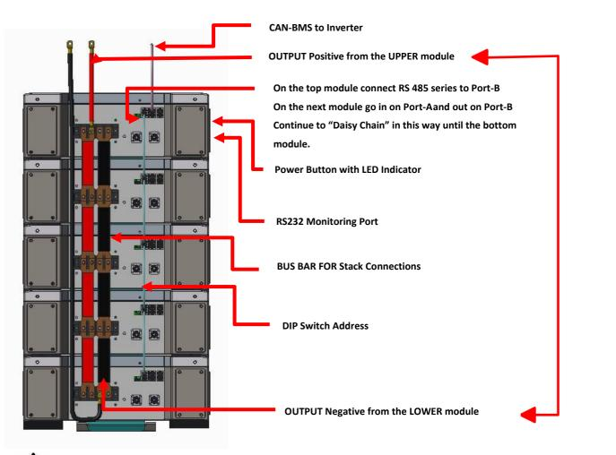
**Information:** When multiple battery boxes are connected together is possible to choose between "capacity" chain series or parallel to increase capacity and peak. In case of parallel the parallel battery and inverter can only communicate through CAN interface, and the communication between the batteries will be through RS485
