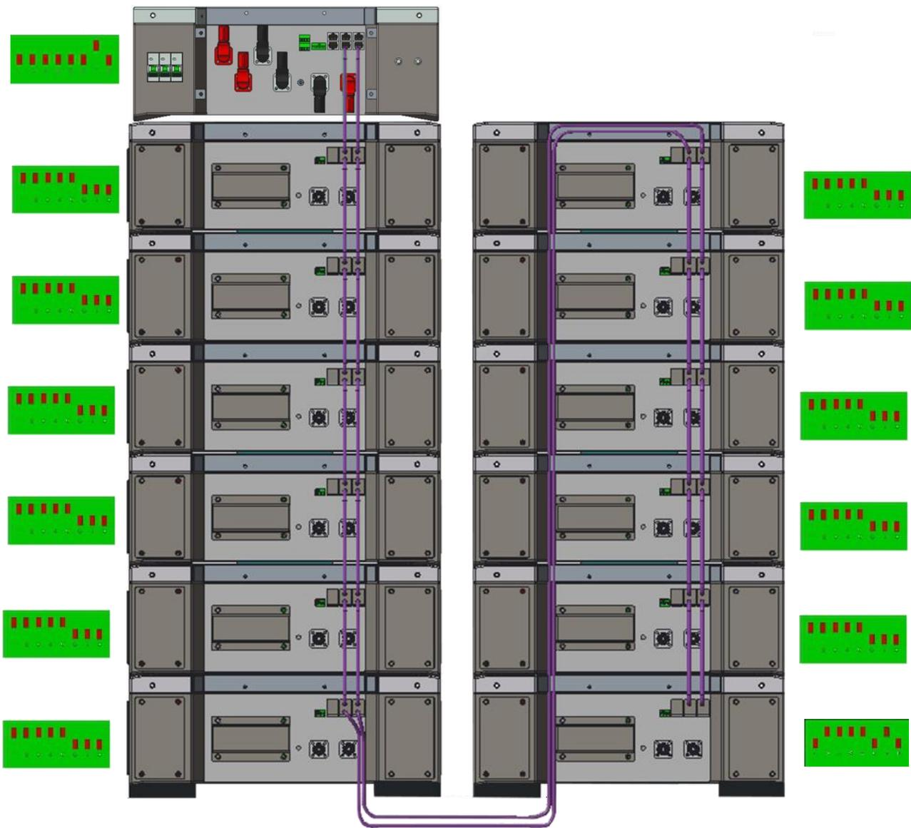
**Step 4:** Link all modules and the HV box with a 6mm Ground cable ( In/Out) by using the GND connections point
