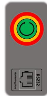
A 2-second press on the Power Button will turn the battery module on.
