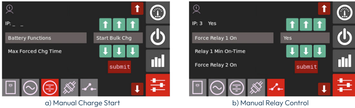
Figure 24. The battery control and relay control screens.
