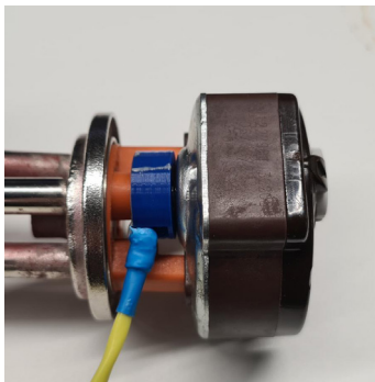
Figure 6. Temperature Sensor Installation
