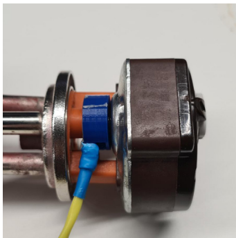
Figure 6. Temperature Sensor Installation
