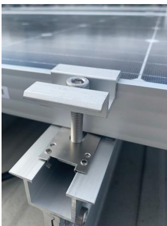
Figure 2 ASCENT Kliplok mounting using the mid clamp to clamp 2 panels and the end clamp to clamp the panels at the end of a string
