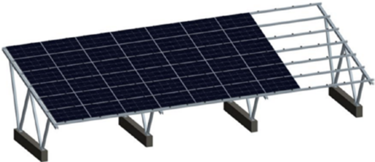
Figure 2. ASCENT mounting structure for IBR roofing sheets
