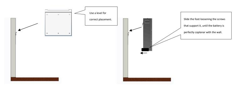
Step 3: Attach the support plate to the wall.
