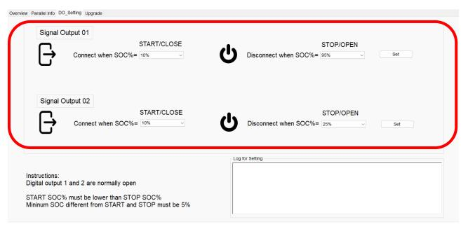
DO1 and 2 dry contacts (Digital Output 1 and 2) are two normally open contacts, which can be set to close within a user-defined range by setting the closing and opening threshold.
