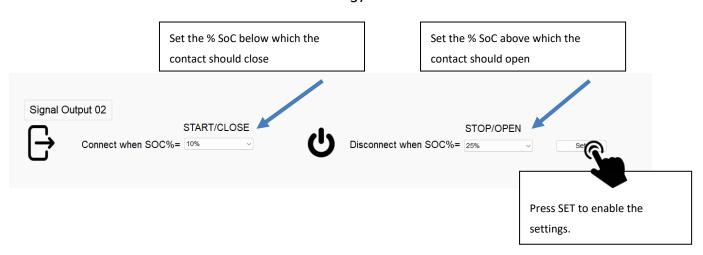
The thresholds can be set freely in the range between 0% and 100%, respecting the following rules:
