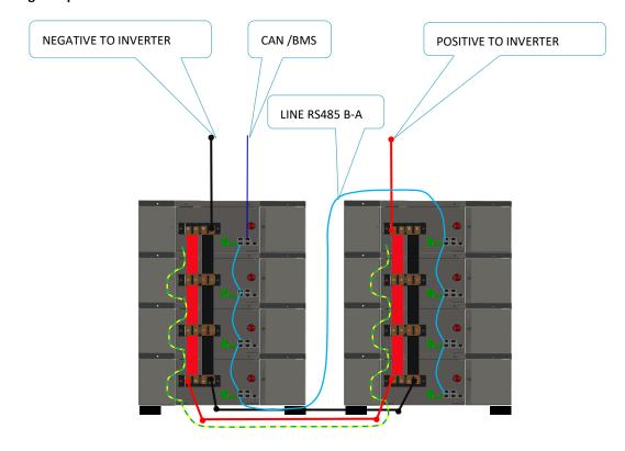
After all cables and bar buses have been connected and the inverter has been set correctly, place the rocker switches (see section 5.4) of all batteries on ON (I). Try to start the system by turning on only the master module: if the installation is set correctly all modules will turn on in sequence.
