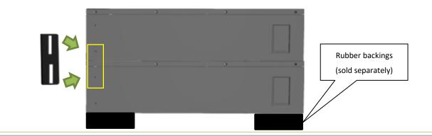
Step 4: Once each battery has been installed horizontally, the feet supplied with the battery in standard configuration can be removed and installed through the modules to constrain the modules on both sides.
