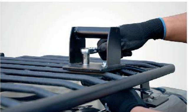
Place the Holding plate (B) below the Base plate (A). Insert washers (D) and bolts (C) in the base plate holes, then, inserting washers (D) and nylon lock nuts (E) in the bolts (C).
