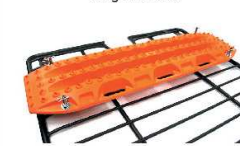
Maxtrax mount for the floor of tubing and mesh racks
