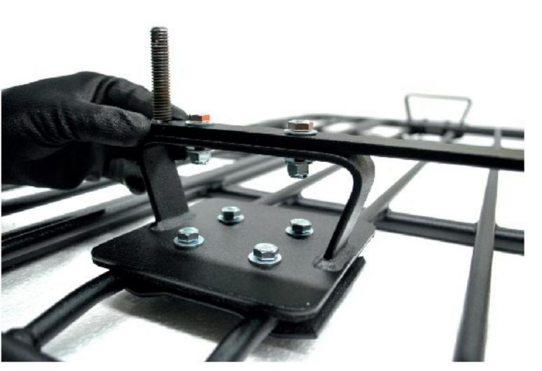
Note: Apply grease (L) to bolt threads before adding nuts and tightening. For Maxtrax Flat Support plate (A), has a preassembled hardware (D, E, F). Don't loosen bolts and nuts, is not necessary!.
