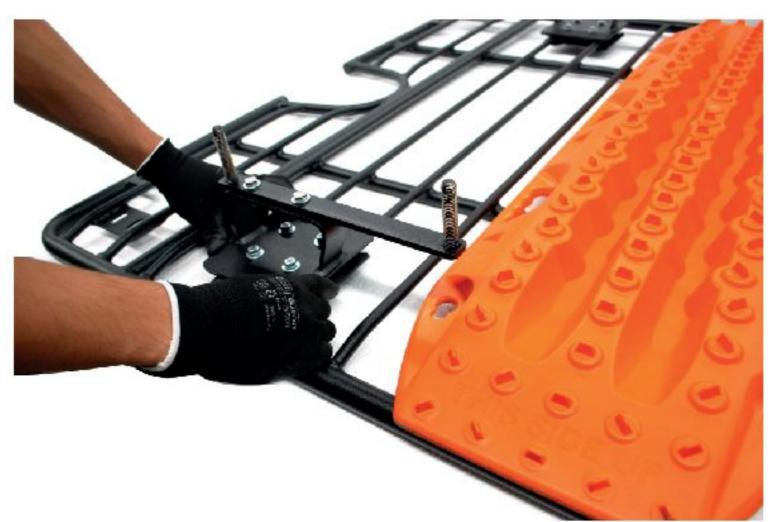
Tighten with 9/16" wrench & ratchet. Repeat steps 1 to 3 for the second Maxtrax mount.
