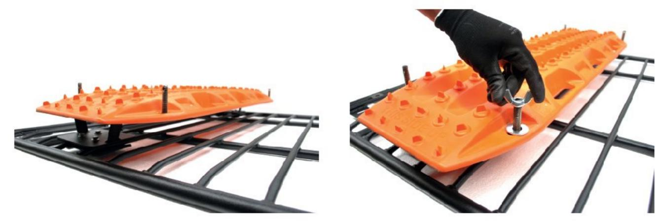
Note: It's recommendable using grease (J) on Maxtrax Flat support plate bolts, and then insert outer washer (G) and wing nut (H).
