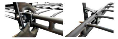
Adjust Mxt-b (B) and add Washer (F) with Lock Nylon Nut (K). Tighten with 9/16" wrench
