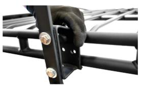
Place Mxt-b (B) on the opposite side of the lateral and add Washer (F) and bolt (C).
