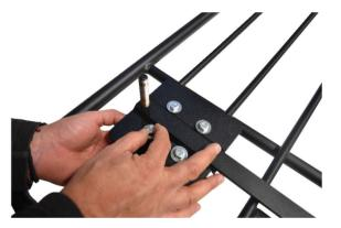
Place the Maxtrax on bolts and add Outer Washer (F) and tighten Wing Nut (G) for each bolt. Insert lock pin (H) in each bolt.
