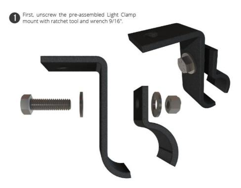
Place the Light Clamp A (A) support on anywhere you want as long as it's a 1" tube, then place the Light Clamp B (B) on the rear and insert washers, bolts and nylon lock nuts. You will need to tighten carefully the bolt and nylon lock nut with ratchet tool and wrench 9/16".
