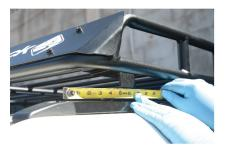
Finally, tighten all roof bolts to the recommended torque 55 in-lb. You can try 13mm or 1/2"wrench or socket.
