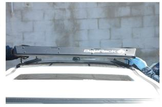
To position the rack in the right place use a tape measure, the distance between the front bracket and the front roof rail should be 5".
