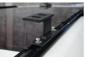
Note: Remember to apply grease (F) to the threads of the bolts.
