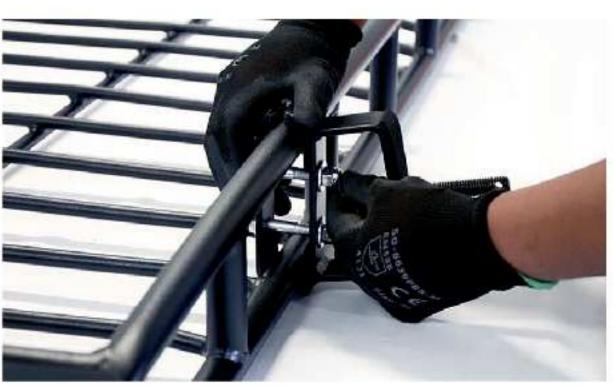
Place the Holding plate (B) on the rear of the side and insert the bolts (D) with washers (E) thorugh the holes and then place the washers (E) and nylon loc knuts (F). See the top image as reference.
