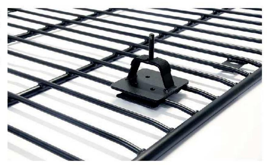
Insert 4 bolts (D) with washers (E) through the HLA mounts holes and the then place the secure plate (B) below of the floor of the rack. Add nylon lock nuts (F) and washers (E) and tighten with the hands.
