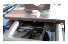
**3** Repeat step 1 and 2 for other mounts and adjust the mounts according to your accessory, tighten the bolts with a 5/16" wrench and 5/16" ratchet tool.
