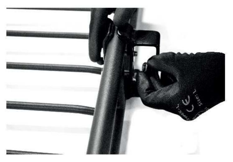
Insert washers (D) with the locknuts (E) in bolts and tighten. Repeat process for other side.
