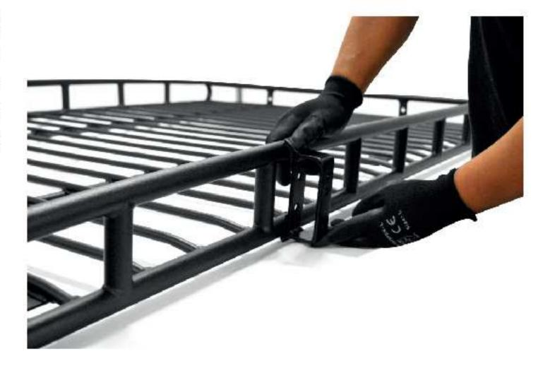
Once you have determined an appropriate location for your base mounts, attach the holding plate (B) on the rear and insert bolt (C) and washer (D) as shown above photo.
