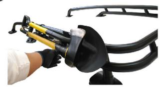
6 Insert secure plate (C) in bolts of Ashovel mounts. Insert washer (G) and wing nut (I) and tighten with hands. Then insert lockpin as shown in above photo. Repeat for other Ashovel mount.
