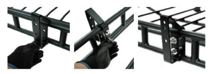
NOTE: Remember to add some GREASE over threads of bolts before inserting in nylon lock nuts. Do not tighten completely because you will have to adjust the mounts.
