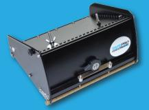
The Tapepro T2 Flat Boxes are designed to apply joint compound to all flat recess and butt joints, automatically crowning the joint and feathering the edges. The coat thickness is controlled by a cam adjuster on the front of the box; more spring pressure results in a lighter coat.
