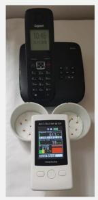
Location (1) EMF (RF) radiation (at 5 cm distance of DEC telephone) = ± 2.780 V/m
