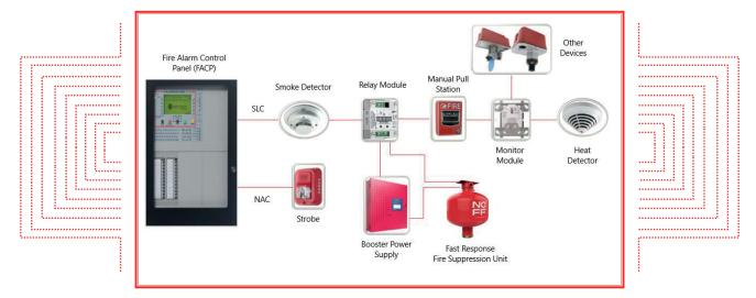
b) Example connection with a Notifier fire alarm and detection system (Automatic means):
