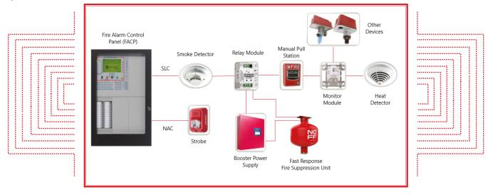
B) EXAMPLE CONNECTION WITH A NOTIFIER FIRE ALARM AND DETECTION SYSTEM (AUTOMATIC MEANS):
