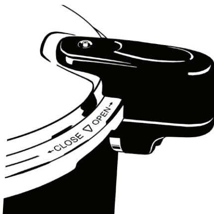
Pressurized and Locked Cover locking pin is lifted
